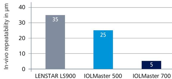
Comparison of the repeatability of axial length measurement<sup>9</sup>
